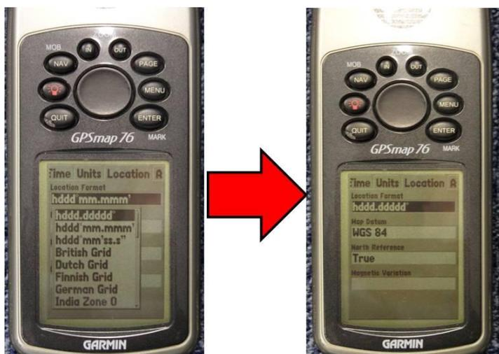
FIGURE 21. In order to harmonize the gathered coordinates with the cartography commonly used, it is recommended to select WGS84 datum and decimal degrees in hddd.dddd° format
