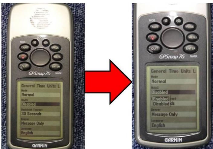
FIGURE 20. WAAS could be ‘Disabled’ when purchasing the GPS receiver. If we want to enhance the accuracy in positioning, it is strongly recommended to make enable this option
