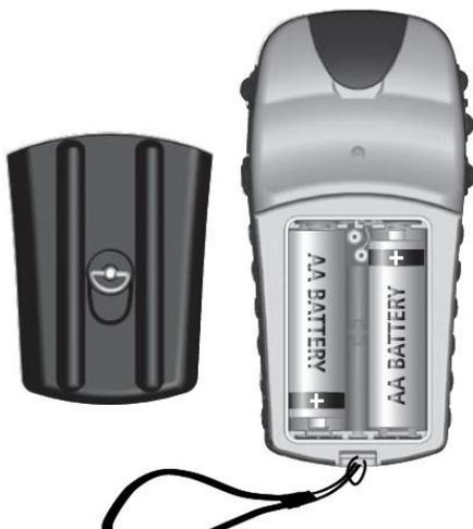
Note: To change the batteries, open the back plastic cover.
